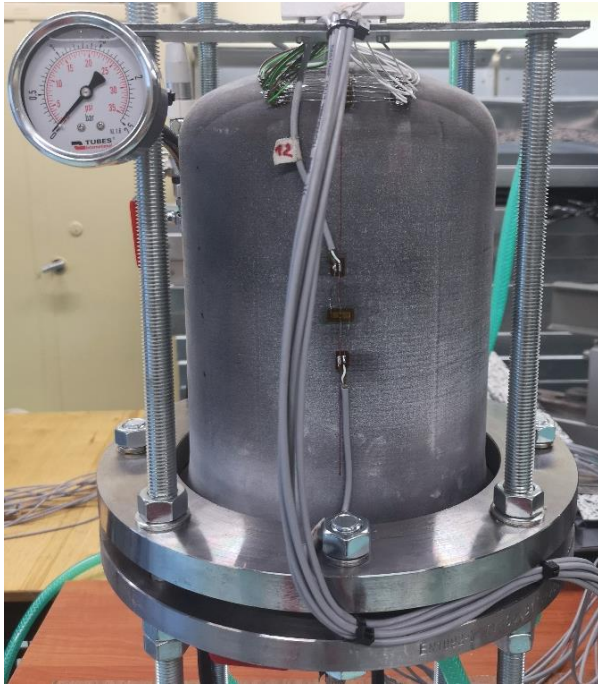
Fig. 7.16. Test bench setup for the pressure vessel with torispherical dished ends
