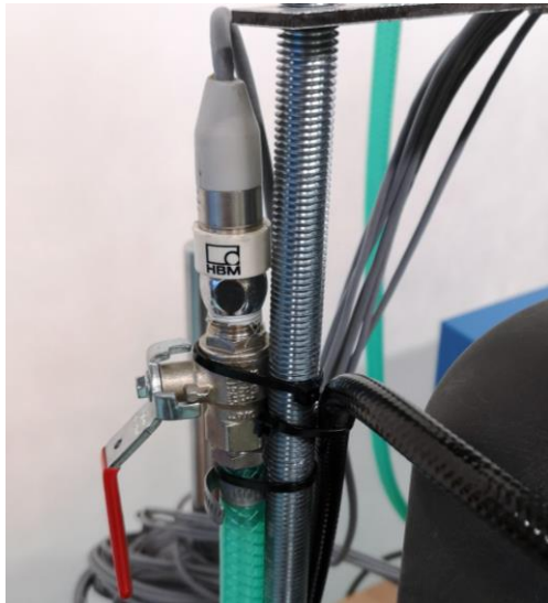
Fig. 7.14. Pressure sensor HBM P8AP
