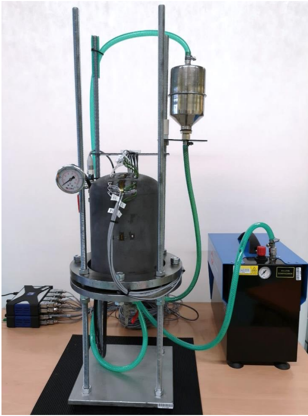
Fig. 7.28. Test bench setup for a pressure vessel with optimized dished end
