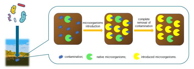
Fig. 10 Schematic presentation of bioaugmentation principle.
