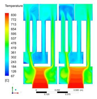
**Fig. 4.** Temperature distribution of flue gas in the XY plane, a) unhampered flow for 30% of nominal power, b) limited flow for 30% of nominal power, c) unhampered flow for 100% of nominal power, d) limited flow for 100% of nominal power.
