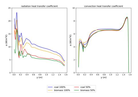
**Figure 8.** Distribution of radiation and convection heat transfer coefficient obtained on the flue gas side of a chamber wall as a function of combustion chamber height.
