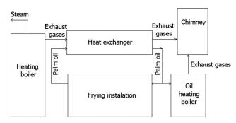
Figure 1. Scheme of a heat recovery plant.
