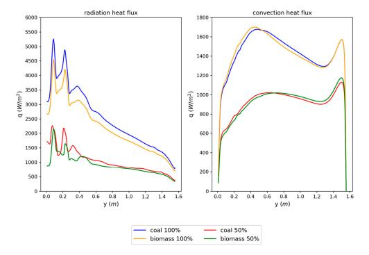
**Figure 7.** Distribution of radiation and convection heat flux obtained on the flue gas side of a chamber wall as a function of combustion chamber height.
