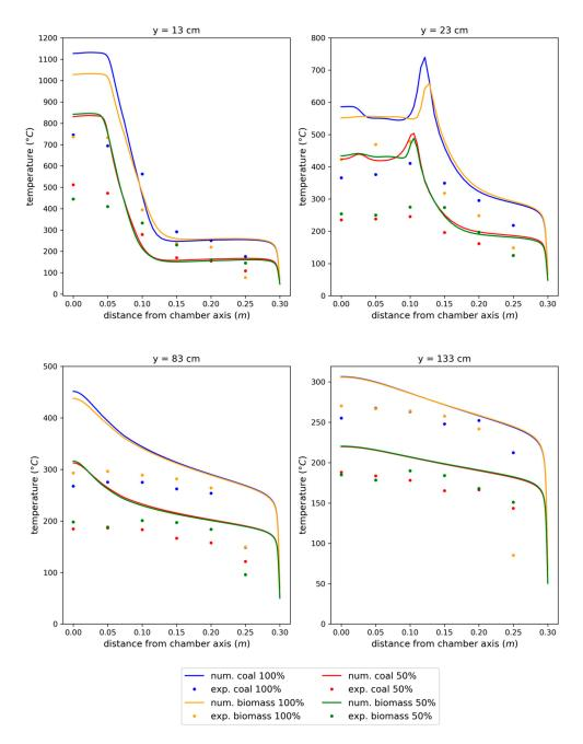
**Figure 4.** Comparison of an exhaust gas temperature distribution at different heights in the combustion chamber obtained from an experimental and a numerical part of the research.
