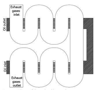
Figure 2. Scheme of the analyzed heat exchanger.
