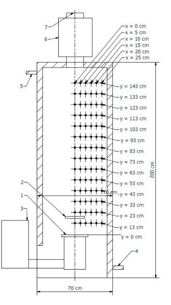
**Figure 1.** Scheme of a cylindrical chamber with marked measurement points used during the experiment, 1—retort feeder, 2—deflector, 3—fuel tray, 4—water inlet, 5—water outlet, 6—insulated measurement duct, 7—flue gas outlet to the chimney.
