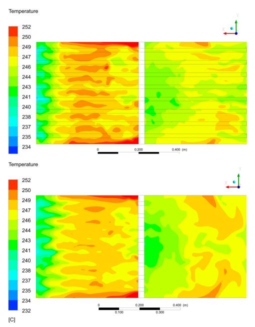
Figure 12. Temperature distribution obtained in the cross-section located after 6 (upper) and 8 rows (lower) of pipes along to the flow in the shell side.
