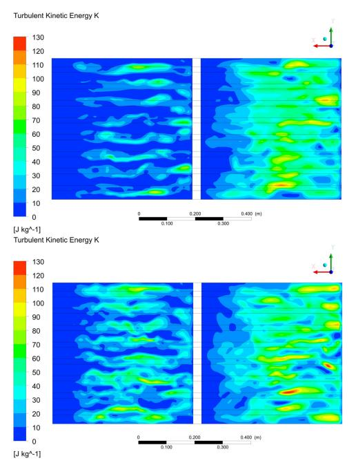
Figure 13. Distribution of turbulent kinetic energy obtained in the cross-section located after 2 (upper) and 4 rows (lower) of pipes along to the flow in the shell side.
