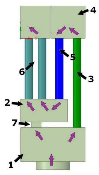
**Fig. 3.** The operation scheme of heating boiler work, 1 – combustion chamber, 2 – afterburning chamber, 3 – first draught, 4 – reversing chamber, 5 – second draught, 6 – third draught, 7 – channel connecting combustion and afterburning chambers.
