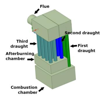
Fig. 2. Draughts location in the heating boiler structure.
