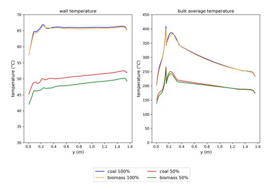
**Figure 5.** Distribution of exhaust gas temperature located in a layer neighboring with the combustion chamber wall and a bulk area-average temperature of flue gas as a function of chamber height.
