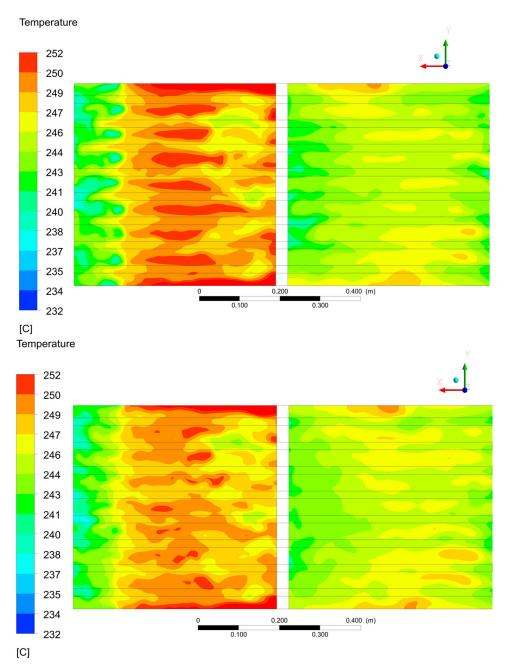
Figure 11. Temperature distribution obtained in the cross-section located after 2 (upper) and 4 rows (lower) of pipes along to the flow in the shell side.
