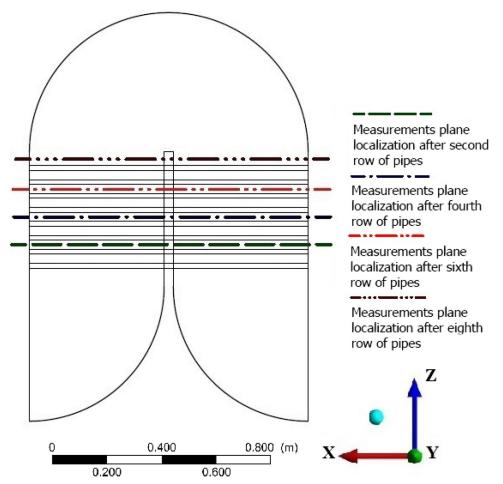
Figure 10. Location of measurement planes for analysis of the character of a fluid realized between the bank of tubes in analyzed sections of heat exchanger construction.
