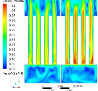
**Fig. 6.** Distribution of amount of exhaust flow through the first draught a) unhampered flow for 30% of nominal power, b) limited flow for 30% of nominal power, c) unhampered flow for 100% of nominal power, d) limited flow for 100% of nominal power.
