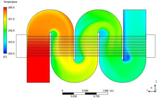
Figure 3. The temperature distribution of exhaust gases for a first module of the heat exchanger.
