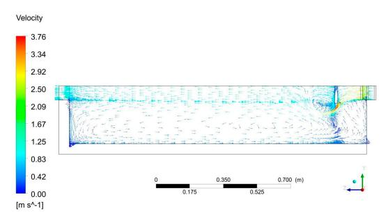
Figure 6. Visualization of the character of a flow inside a combustion chamber.
