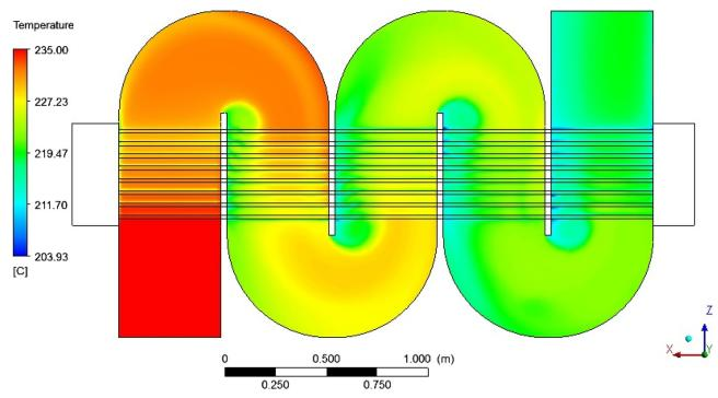
Figure 4. The temperature distribution of exhaust gases in a second module of the heat exchanger.
