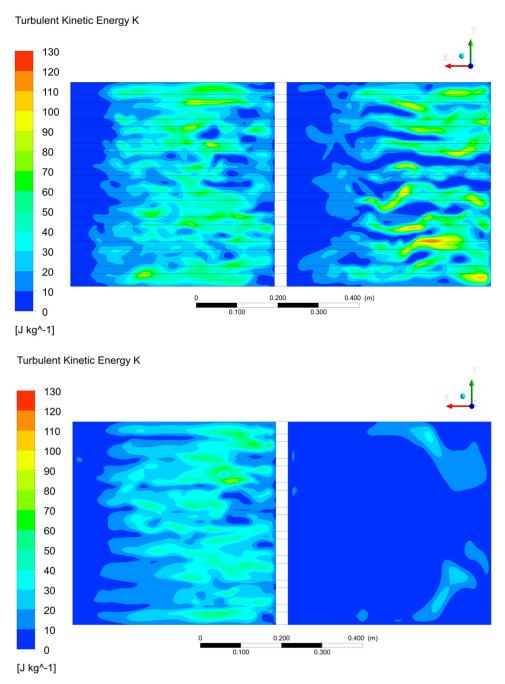
Figure 14. Distribution of turbulent kinetic energy obtained in the cross-section located after 6 (upper) and 8 rows (lower) of pipes along to the flow in the shell side.
