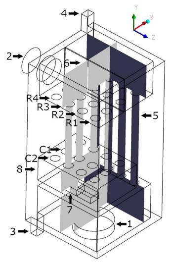
**Fig. 1.** Construction of the heating boiler with marked crucial planes (XY and YZ) used in results analysis, 1 – combustion chamber, 2 – flue, 3 – water inlet, 4 – water outlet, 5 – plane YZ, 6 – plane XY, 7 – directly connection between combustion chamber and the afterburning chamber, 8 – afterburning chamber, C1-2 – lines of pipes in the draught, R1-R4 - rows of pipes in the draught.
