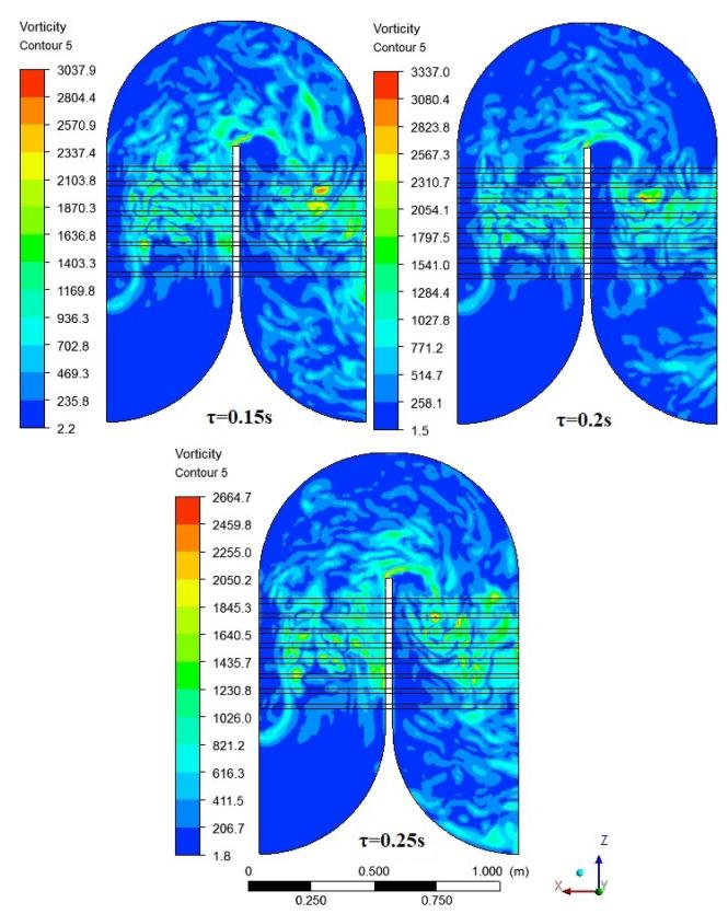
Figure 8. Distribution of vorticity for one of the sections of heat exchanger obtained for three different time steps.
