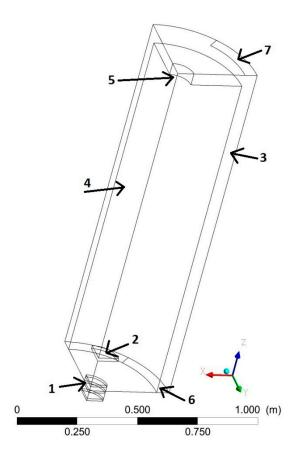
**Figure 3.** Overview on a computational domain, 1—volume of fixed bed, 2—deflector, 3—water jacket, 4—combustion chamber, 5—exhaust gas outlet, 6—cooling water inlet, 7—cooling water outlet.
