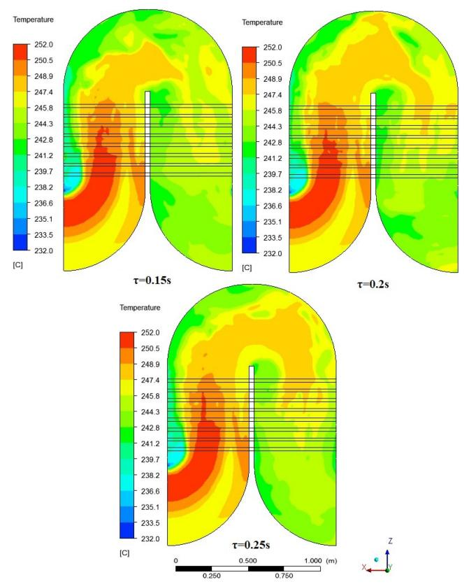
Figure 9. Temperature distribution for one of the sections of heat exchanger obtained for three analyzed time steps.
