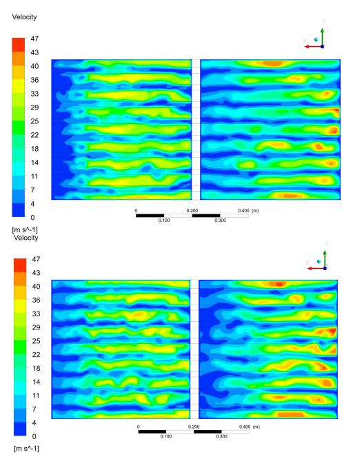
Figure 15. Velocity distribution obtained in the cross-section located after 2 (upper) and 4 rows (lower) of pipes along to the flow in the shell side.
