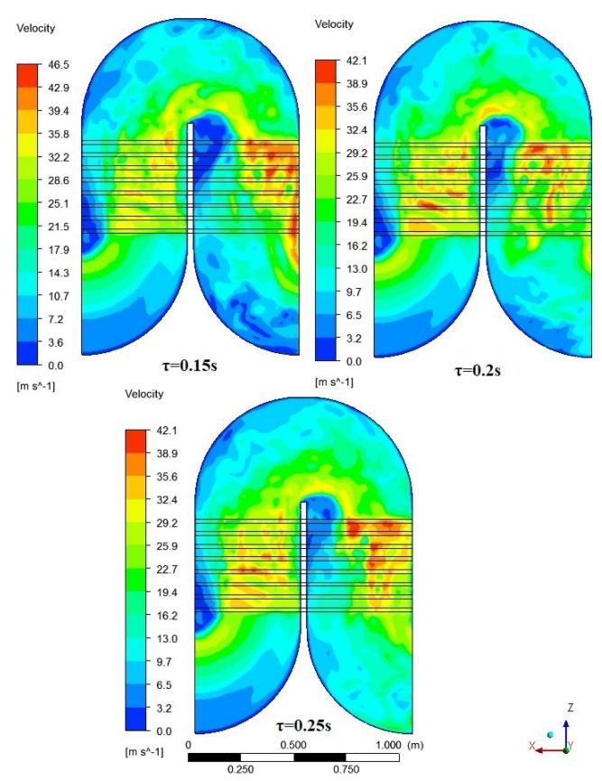
Figure 6. Velocity distribution for one of the sections of heat exchanger obtained for three analyzed time steps.
