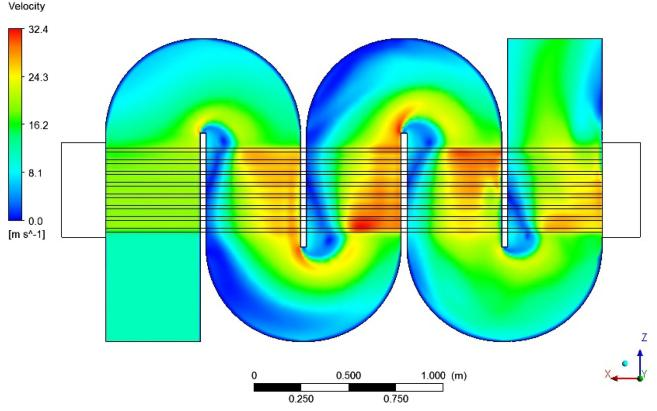
Figure 5. Velocity distribution in a first module of the heat exchanger.
